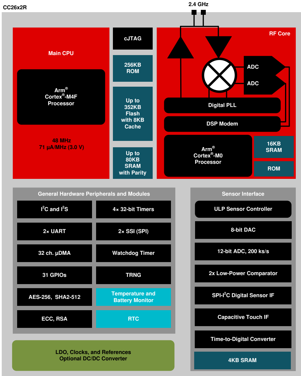
Figure 4-1. CC2652R Block Diagram
