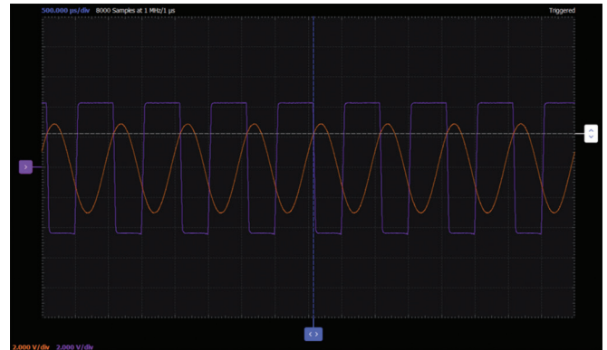
Figure 14. Inverting hysteresis comparator with asymmetric thresholds waveform.
