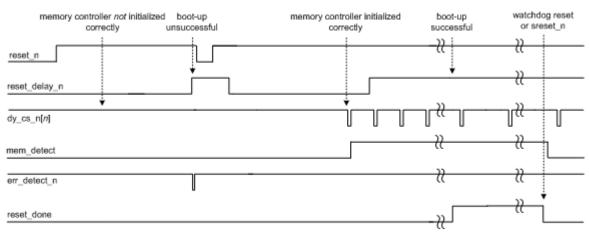
This timing diagram illustrates the recovery process:
